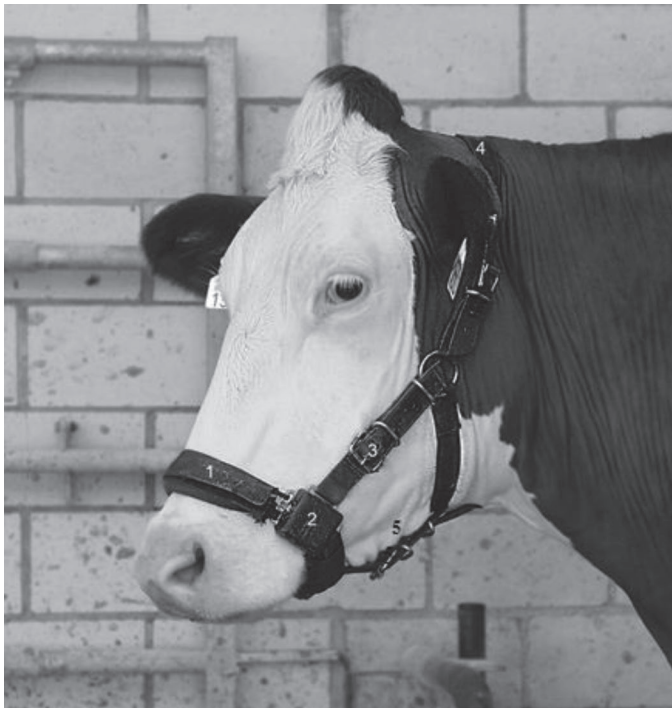
Figure 1. Red Holstein cow wearing a RumiWatch Halter version 6.0 (Itin and Hoch GmbH, Liestal, Switzerland). 1: Belt around the nose including a pouch with a propylene glycol-filled tube and the pressure sensor. 2: Waterproof plastic protection box (left side: battery; right side: triaxial-accelerometer, data logger, and secure digital memory card). 3, 4, 5: Adjustment buckles at the side, on the neck, and under the lower jaw, respectively.
